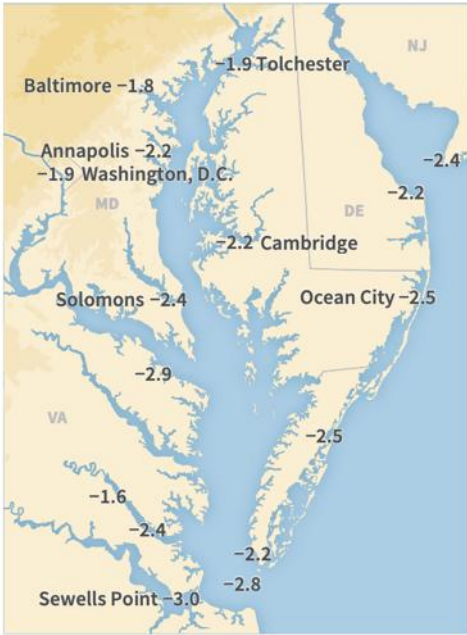
Figure 10. Vertical land motion (mm/yr) estimated by NOAA from tide-gauge records in Chesapeake Bay and adjacent Atlantic coast.
